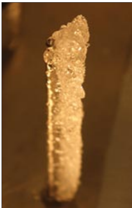
Figure 4. Saturation ice on a modern optical ice sensor probe.
