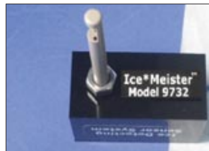
Figure 1. This commercial, off-the-shelf, in-flight ice sensor monitors the optical characteristics of whatever substance is in contact with the optical surfaces of the probe, either air (NO ICE) or water ice (ICE ALERT). Ambient wind blows standing water away, but ice sticks. Made of nonconductive delrin and acrylic plastics, probe is electromagnetically compatible with its host aircraft radio environment, and can be installed in close proximity to radio antennas.
