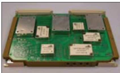
Figure 5. VME power supply built from off-the-shelf DC-DC converter modules.
