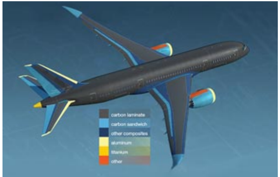
Figure 1. Advanced composites used throughout the Boeing 787 account for more than fifty percent of the aircraft body 1 . (Copyright © Boeing)
